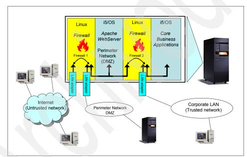
Figure 11-6 i5/OS partitions under control of the firewall
