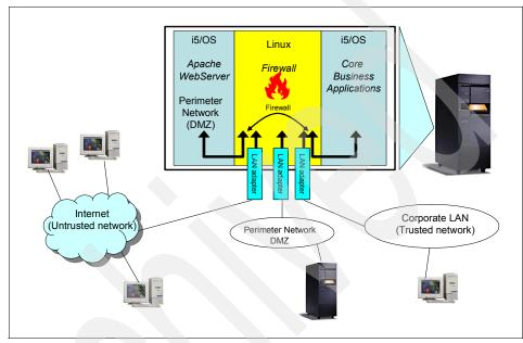
Figure 11-7 System i machine protected by one firewall
