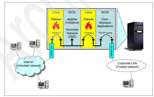
A typical On Demand Business configuration is to use two Linux firewall partitions to create a DMZ as shown in Figure 11-4.
