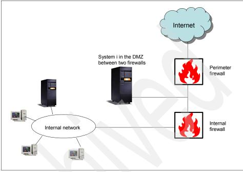
Figure 11-2 shows an example of an environment with two external firewalls and a DMZ between.
