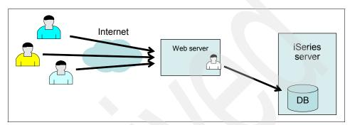
Figure 12-1 Web application accessing a back-end database as a single DB user
