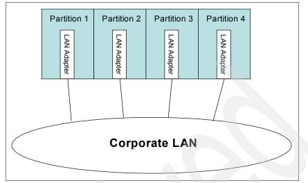
Figure A-3 Interpartition communication with external LAN
