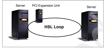
Figure A-4 HSL OptiConnect loop
