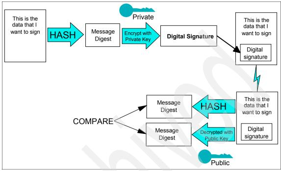
Figure 9-5 shows how the digital signature is used to check the data.
