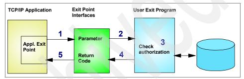
Figure 8-8 Exit program usage example
