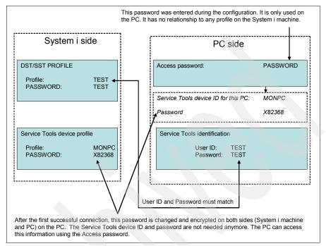
Figure B-3 shows the relationship between profile IDs and passwords during the *connection process* of the LAN console.
