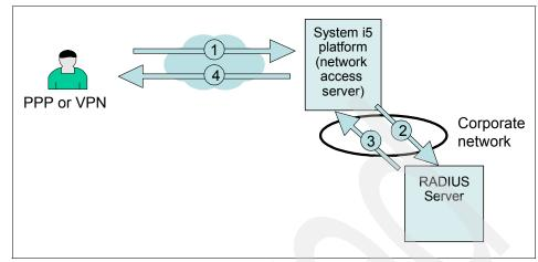
Figure 12-5 Authentication using RADIUS
