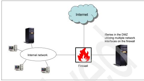
Figure 11-3 Single firewall solution or three-legged firewall solution
