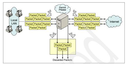
Figure 8-13 IP packet filtering principles
