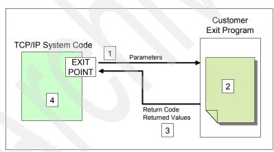
Figure 8-7 TCP/IP exit point processing
