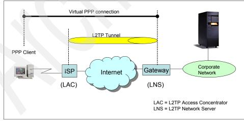
Figure 10-4 L2TP compulsory tunnel
