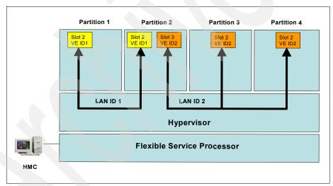
Figure A-6 Virtual Ethernet
