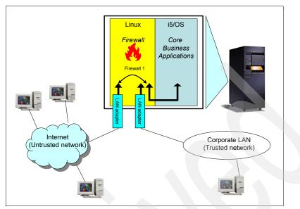
Figure 11-9 Basic configuration of a firewall with a native LAN adapter on Linux
