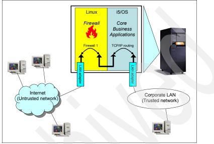
Figure 11-8 Basic configuration of a Linux firewall without DMZ
