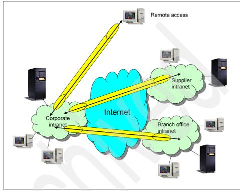
Figure 10-1 shows how VPN connections can be used to connect your remote users through the Internet.
