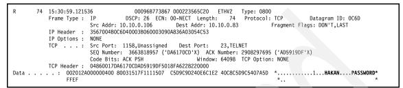
Figure 12-2 User HAKAN with the password PASSWORD captured in a communications trace
