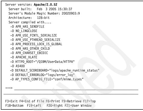
Figure C-3 Displaying the HTTP server (Apache server) version
